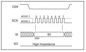
FIGURE 5-6: AUTO ADDRESS INCREMENT (AAI) WORD PROGRAM SEQUENCE WITH HARDWARE END OF WRITE DETECTION
