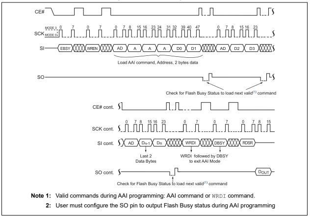
FIGURE 5-7: AUTO ADDRESS INCREMENT (AAI) WORD PROGRAM SEQUENCE WITH SOFTWARE END OF WRITE DETECTION
